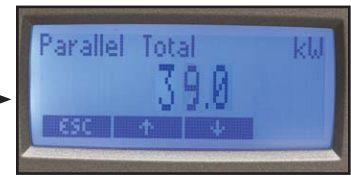
Display full system output from any UPS
