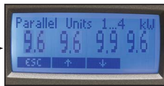
Display output from multiple modules on one screen
